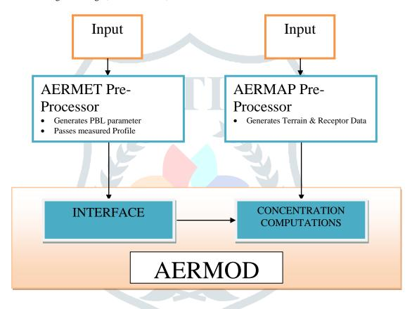
Figure 2: Data flow of AERMOD
