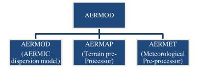
Figure 1: Components of AERMOD
