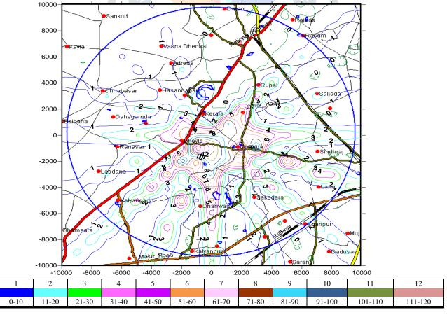
Figure 9: Dispersion of Particulate Matter superimposed on 10 km radius map
