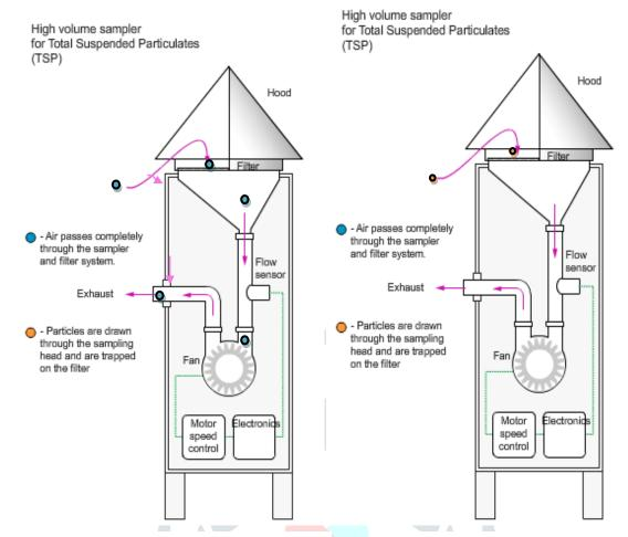
Figure 3: Air Particle gets passed through HVAS
