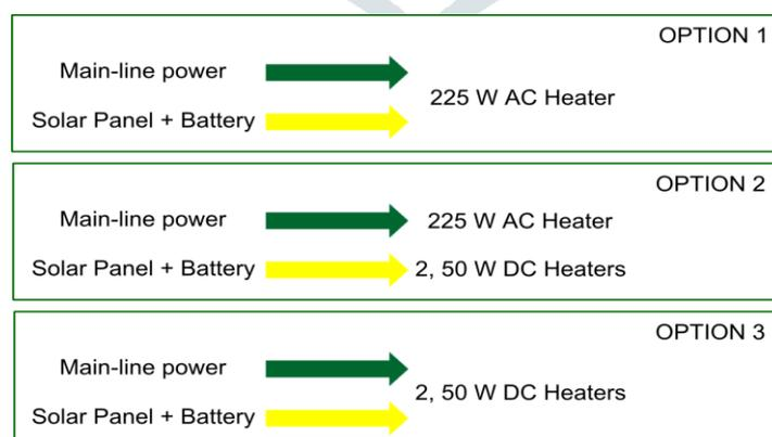
Fig 1: Three heating possibilities are contemplated. The first arrow that is green specifies to the primary supply and the second arrow that is yellow specifies to the secondary supply (used when power grid is not accessible). Here the suitable possibility for the project is possibility or choice 3[2].
