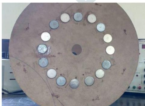
Figure1 – Magnet Arrangement
