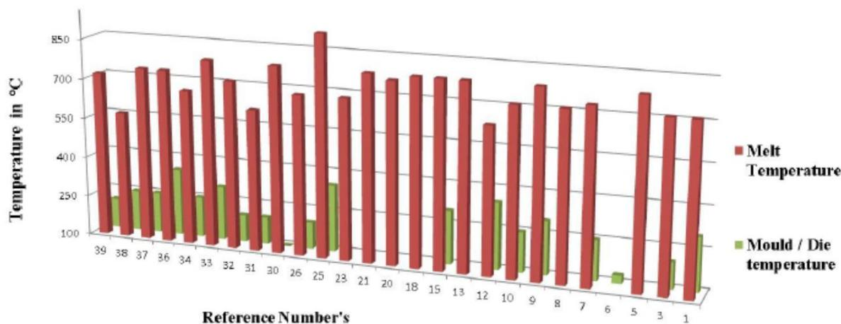
Fig.1 Melting temperature and Die temperature for Squeeze Casting [16]
