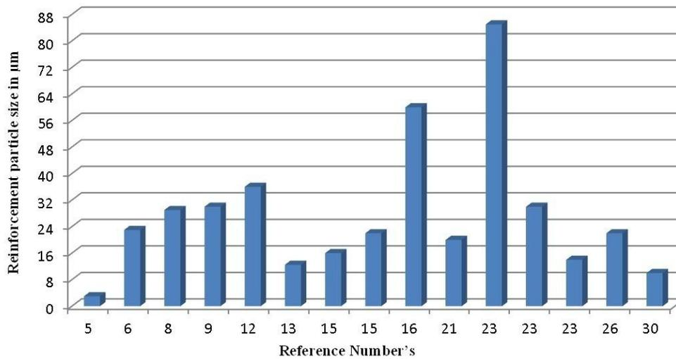
Fig.2 Reinforcement particle size for Squeeze Casting [16]
