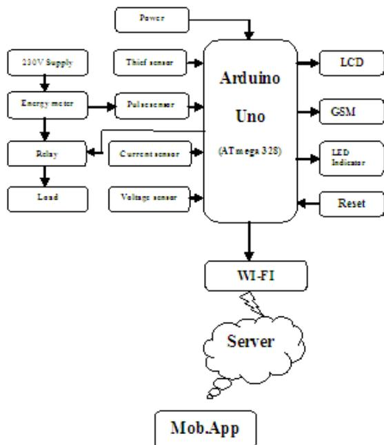
Fig.1. Block Diagram of Smart Energy Meter using Theft Detection For Home Management System
