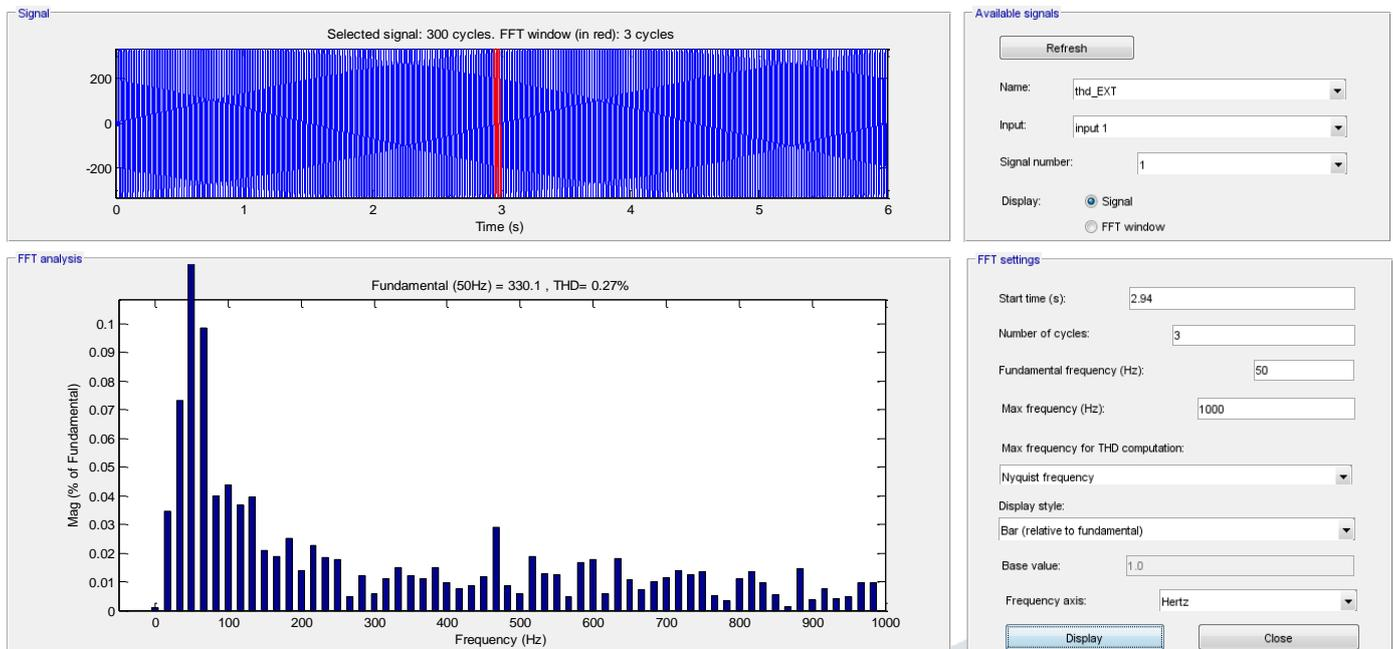
Fig.15.Harmonic spectrum of load voltage.
