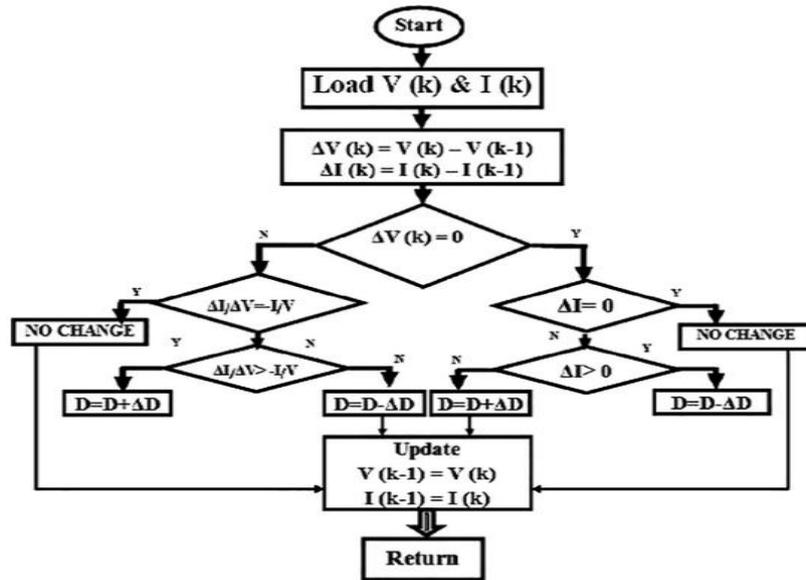
Fig. 5. Incremental Conductance (IC) algorithm for MPPT controller.
