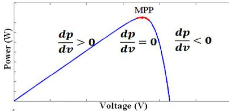
Fig. 4. Operating power (P) and voltage (V) curve of the conventional IC algorithm.
