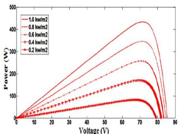
Fig. 3. P-V curve of PV array.
