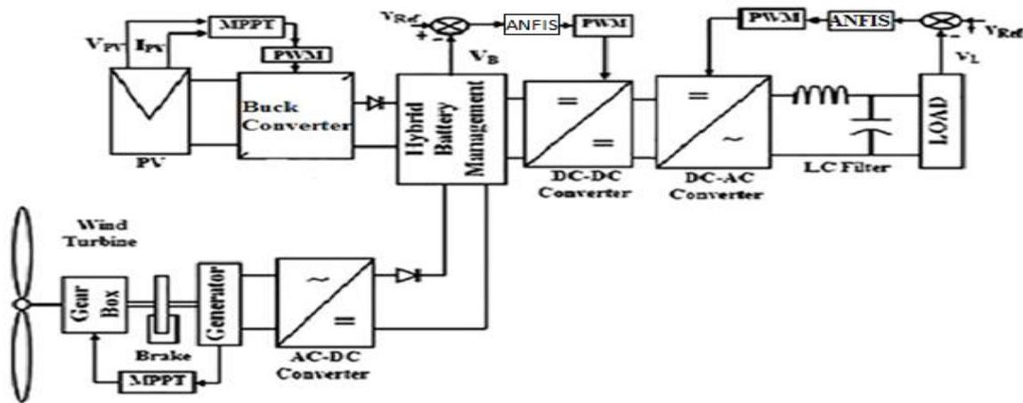
Fig. 1. A standalone hybrid power supply system using solar and wind energy.
