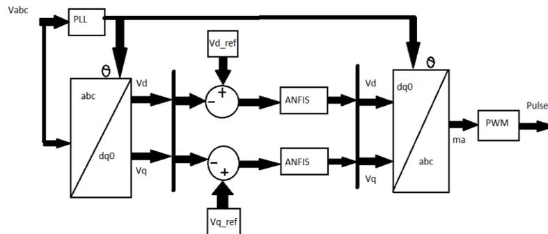
Fig. 11. Block diagram for ANFIS voltage regulator.
