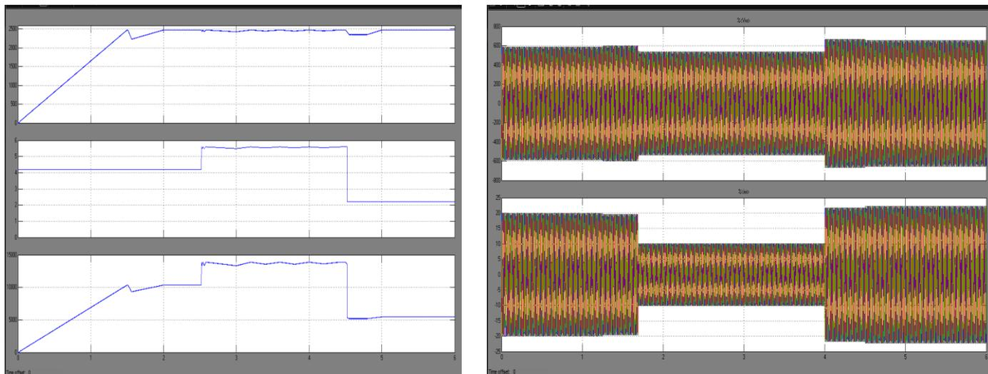
Fig. 12. Generated (a) voltage (b) current (c) power profile of the PV array under variable irradiance of the Sun.
