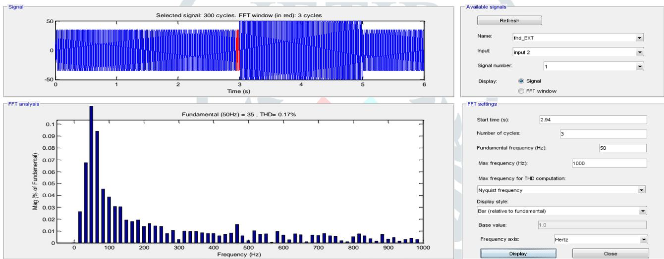
Fig.16.Harmonic spectrum of load current
