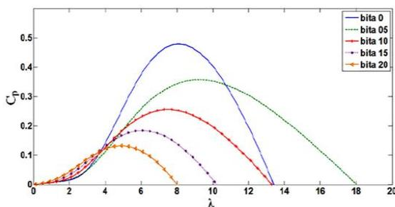
Fig. 6. Analytical approximation of Cp (λ,β) characteristics.
