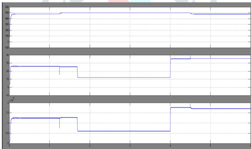
Fig.14.The rectified (a) voltage (b) current (c) power profile of the PMSG connected with WT.
