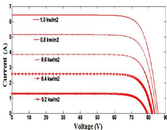
Fig. 2. I-V curve of PV array.
