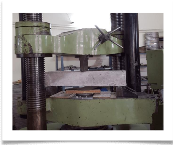
Image 4(b) - Arrangement for loading of flexure test specimen.
