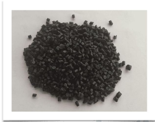
Image 1 - Grinded plastic waste aggregates
