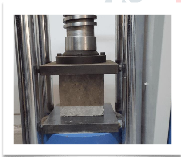
Image 4(a)- Fitting the cube in the compression test machine.
