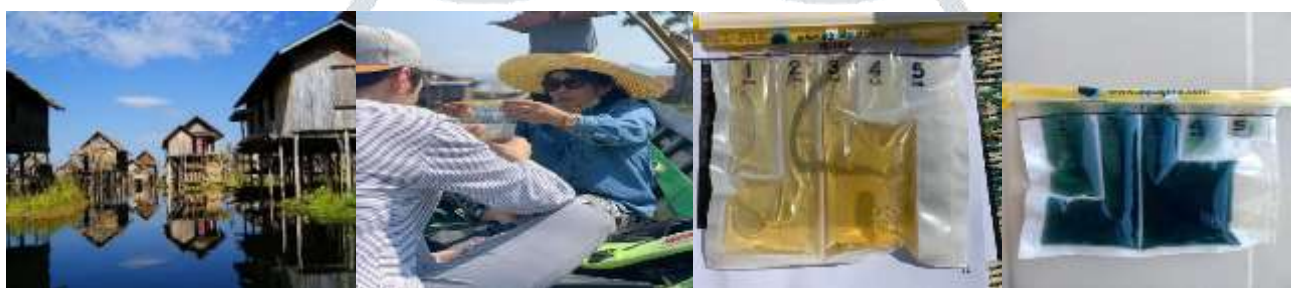
Fig.12 E-coli measurement within Kela village (source: water quality measurement working together with Robbert De Lange from Delft University of Technology, The Netherlands) The result is that the water contains >100 MPN/100 mL, which means highly contaminated water with high health risks.
