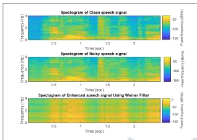
Fig. 6: Spectrogram of Noisy and Enhanced Speech for SNR=5 dB
