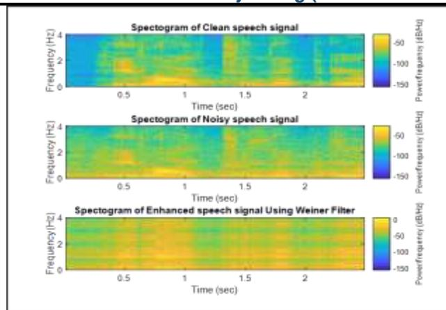
Fig. 8: Spectrogram of Noisy and Enhanced Speech for SNR=5 dB
