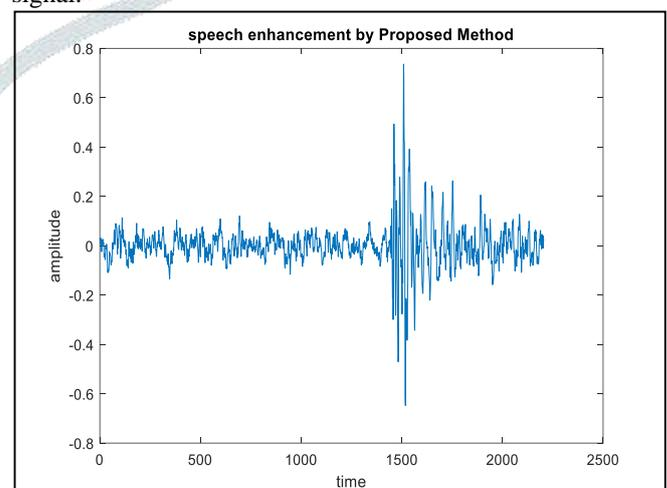
Fig. 5: Speech Enhancement of Signal by Proposed Method
