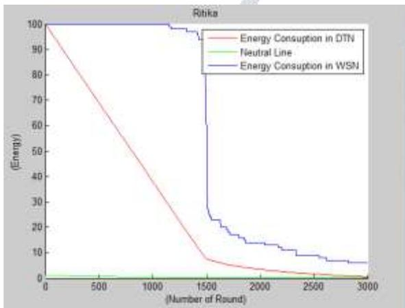
Figure 8: Energy vs. number of rounds of Energy Consumption in DTN, Natural Line, and Energy Consumption in WSN
