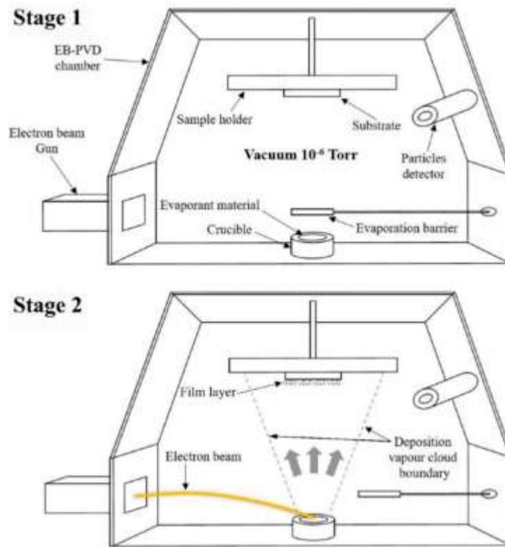
**Figure 3. Schematic of electron beam physical vapor deposition (EB-PVD) equipment (Stage 1) and the generation of the film for coating**
