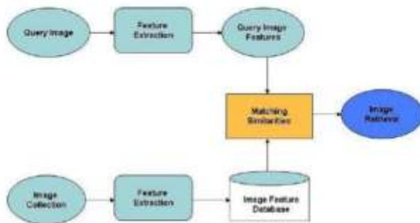
Fig.1 Content Based Image Retrieval Systems
