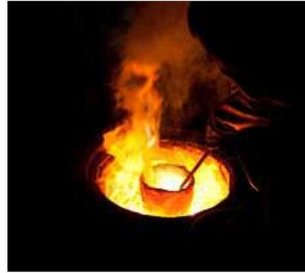
Melting metal in a crucible for casting
