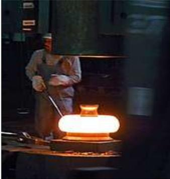
In open die forging hammer strikes on the work piece which is kept on anvil and the deformation takes place. The surfaces are not in contact with each other means the melted metal flows freely unless covered with dies.
