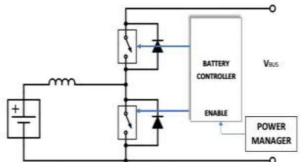
Fig 3: DC-DC Bi-directional Buck-Boost Converter connected to Battery
