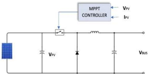
Fig 2: DC-DC Buck Converter connected to the First Stage
