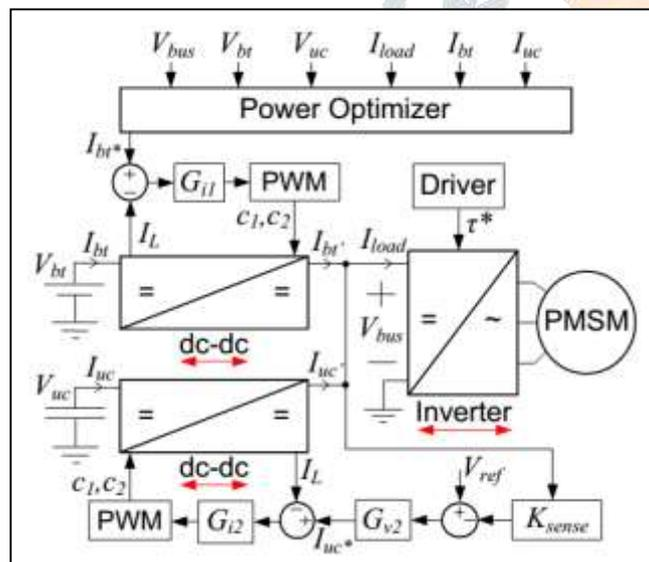
Fig 1: Structure Model of HESS
