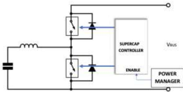
Fig 4: DC-DC Bi-directional Buck-Boost Converter connected to Supercapacitor
