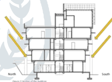
Figure 15 PTM ZEO's self-shading form (Bhattacharyya, 2019)
