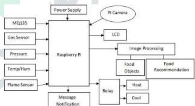
**Description:** Raspberrypi –acts as a microcontroller to perform the multiple operation to measure the food quality. DIP/ DL – digital image processing, it is used to
