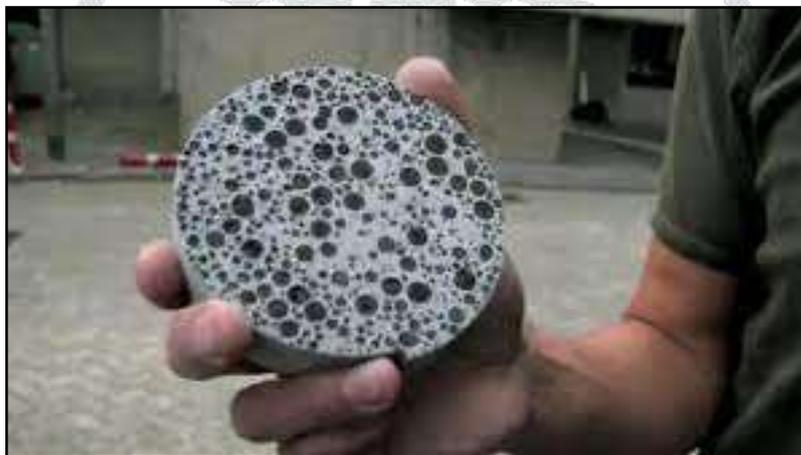
the substantial blend. At the point when breaks show up, the cases separate, delivering the synthetic substances which, when responded with the calcium hydroxide in the substantial, structures a gel which fixes the breaks.
