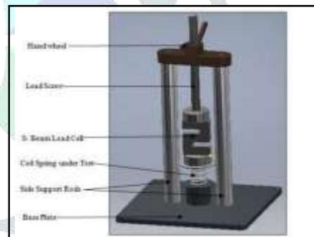
Fig. CAD model of setup
