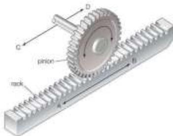
A rack and pinion is a type of linear actuator that comprises a pair of gears which convert rotational motion into linear motion. A circular gear called "the pinion" engages teeth on a linear "gear" bar called "the rack"; rotational motion applied to the pinion causes the rack to move, thereby translating the rotational motion of the pinion into the linear motion of the rack.
