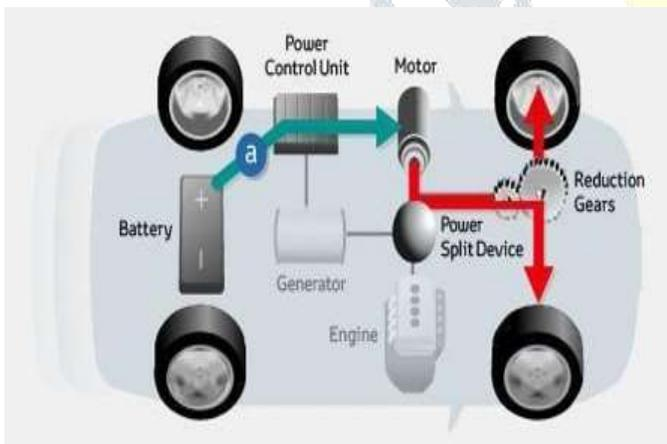
The electric vehicle is driven by the battery. On switching the car the motor takes current from the battery. The motor converts the electrical energy into the mechanical rotation and hence the vehicle moves forward when the car starts running then generation takes place. The synchronous generator
