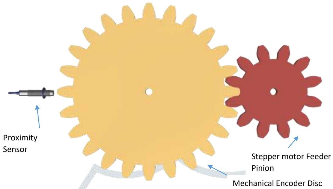
Fig-2 Proposed design Mechanical Encoder
