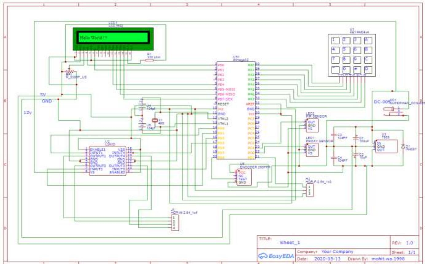
Fig-1 Proposed automatic wire feeder and cutter circuit diagram
