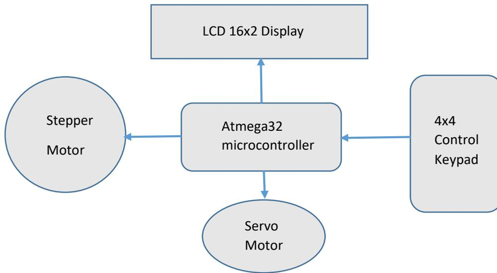
Fig-4 Proposed block diagram of working design
