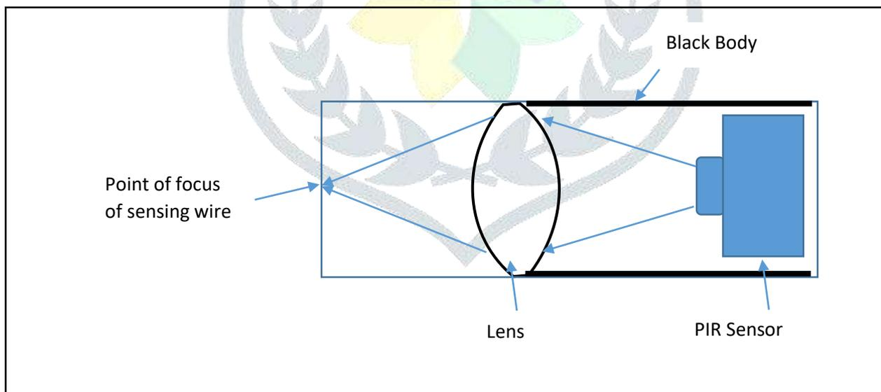
Fig-3 Proposed design Special arrangement PIR Sensor
