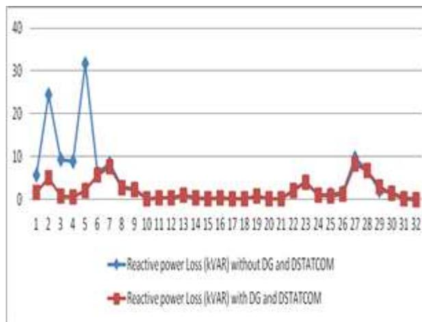
Figure 8 (b). Reactive power losses of IEEE 33 bus RDS
