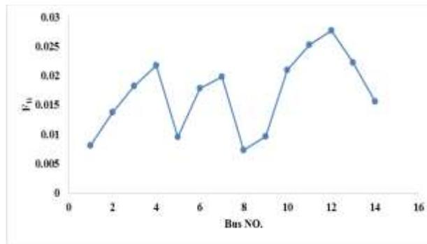
Figure 4. Optimal placement of DG from the 1st objective function is at bus '12'
