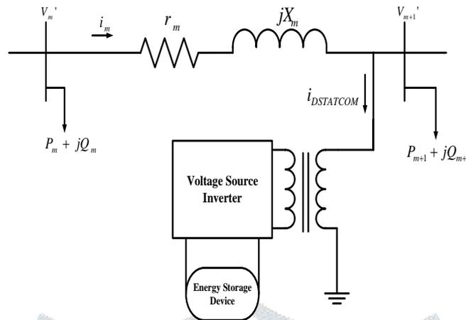
Figure 2. Two bus representation with DSTATCOM [1]
