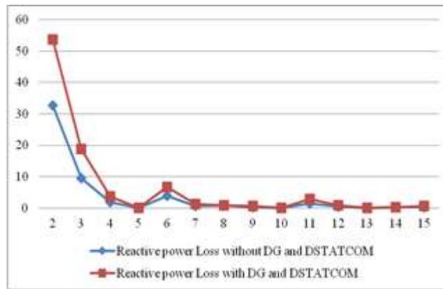
Figure 6 (c). Reactive power losses of IEEE 15 bus RDS
