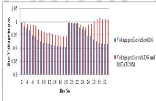
Figure 7. Voltage Profile of IEEE 33 Bus RDS
