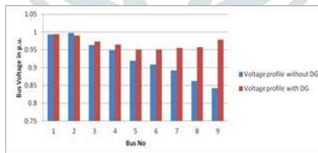
Figure 3. Voltage profile of IEEE 9 BUS RDS
