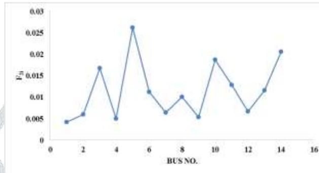
Figure 5. Optimal placement of DG from the 2nd objective function is at bus '5'
