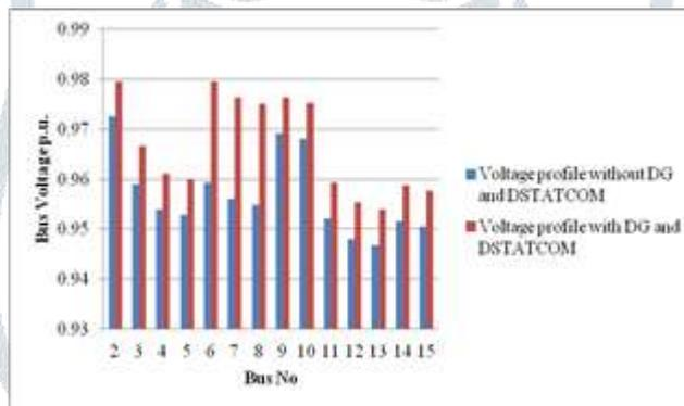
Figure 6 (a). Voltage profile of IEEE 15 bus System
