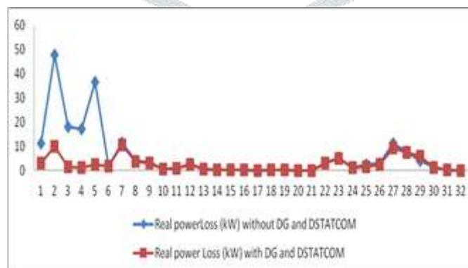
Figure 8 (a). Active power losses of IEEE 33 bus RDS
