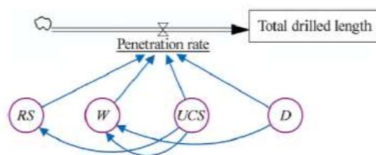
Figure-1 Penetration Rate Of Drilling
