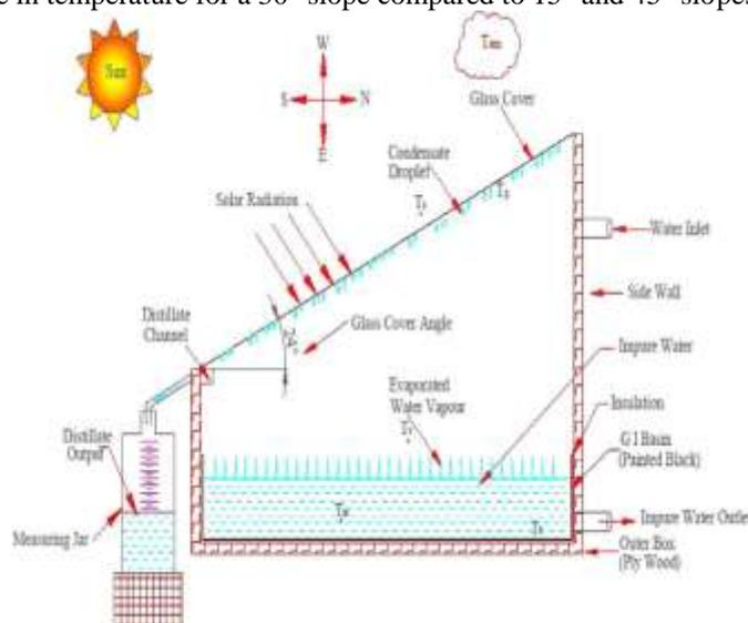
For places with latitude higher than 20, single slope still is preferable. For north latitude places the single slope still with south facing cover and for south latitude places, still with north facing cover are used (Fath et al 2003) [10]. If the double slope still is used for higher latitude places, only one side of the cover will receive the sun rays and other side will be on the shadow side for sun rays.
