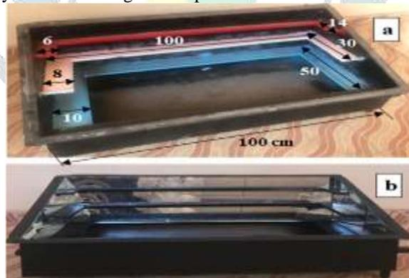
The tray solar still with internal reflector had a distillate more than the reference distiller. Its because of the high evaporation caused by the evaporative surface area of the tray distiller compared to that of the traditional distiller.
