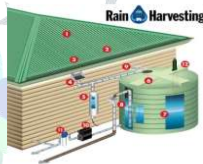
Figure 13: Flow diagram of rain harvesting system and connection with water supply channel
