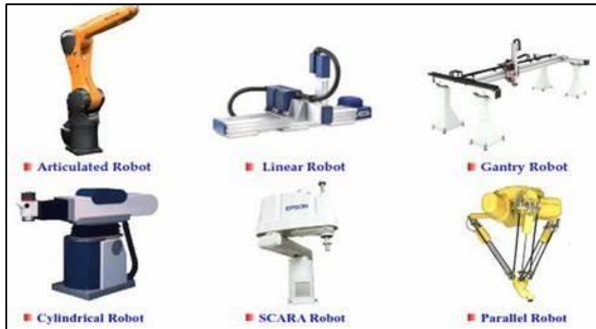
Fig. 2: Different types of robots
