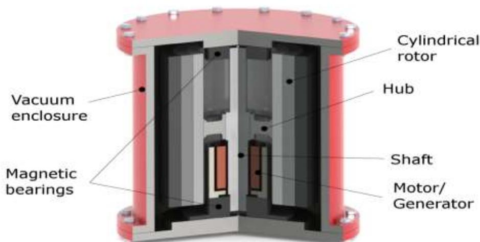
*Figure 1. The main components of a typical flywheel*
