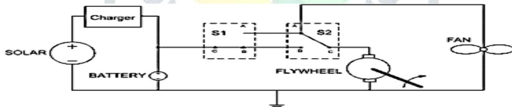
*Figure 2: Schematic Drawing of DC Load System*
