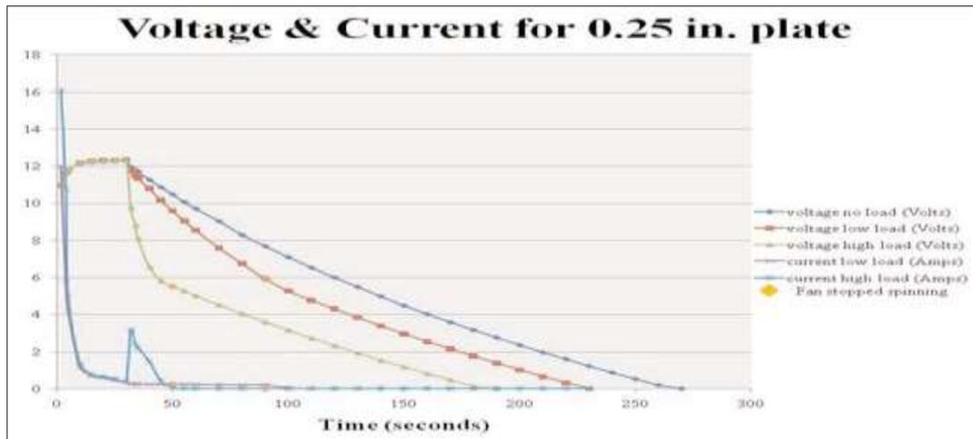
Figure 3: Scatter plot showing averaged voltage and current values vs. time for all load settings for 0.25 in. plate.
