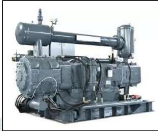
**Figure 2: Double Acting Compressor**
