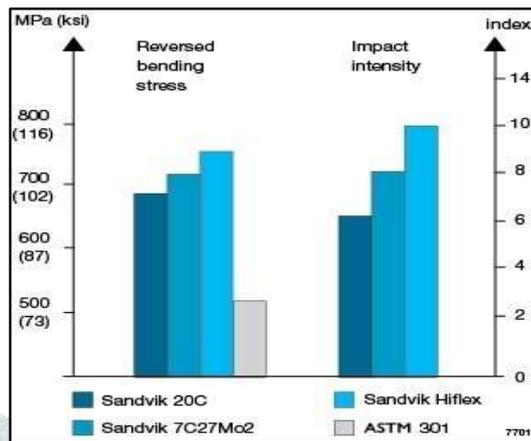
**GRAPH 1: Comparison of fatigue properties for Sandvik's flapper valve steels and standard spring steel (ASTM 301)**
