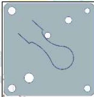
**Figure 5: CAD Model of Flapper Valve**
