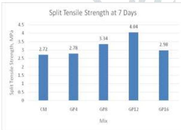
Figure 4. Split Tensile Strength Test Results at 7 Days.
