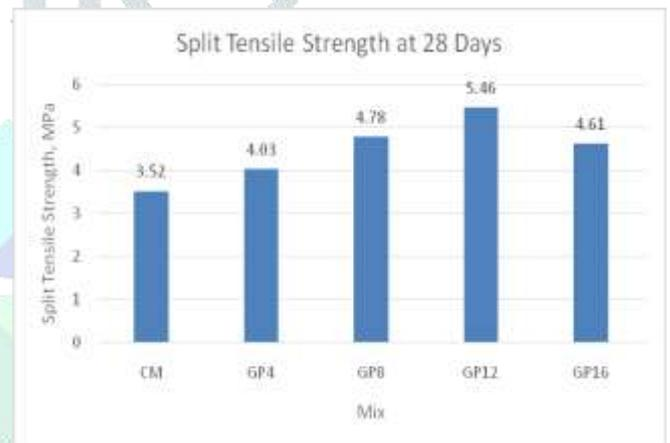
Figure 5. Split Tensile Strength Test Results at 28 Days.
