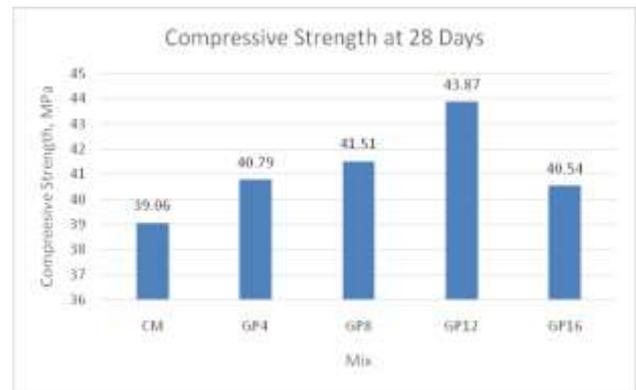
Figure 3. Compressive Strength Test Results at 28 Days.
