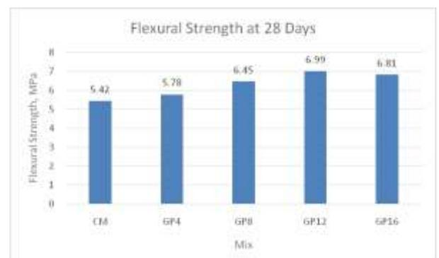
Figure 7. Flexural Strength Test Results at 28 Days.
