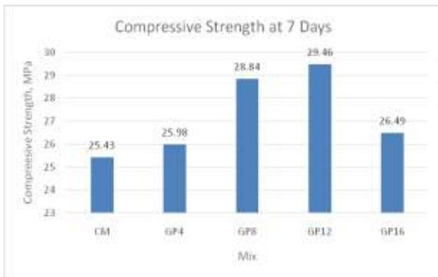
Figure 2. Compressive Strength Test Results at 7 Days.
