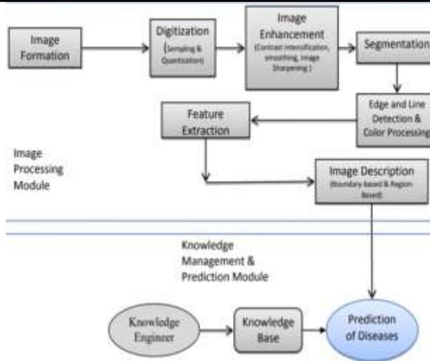
Fig.1- The steps of processing and analysis by the system.
