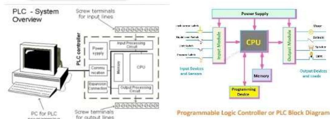
PLCs are complex and powerful computers; it takes inputs, performs logic on the inputs in the CPU and then turns on or off outputs based on that logic. We can take the following case for example:
