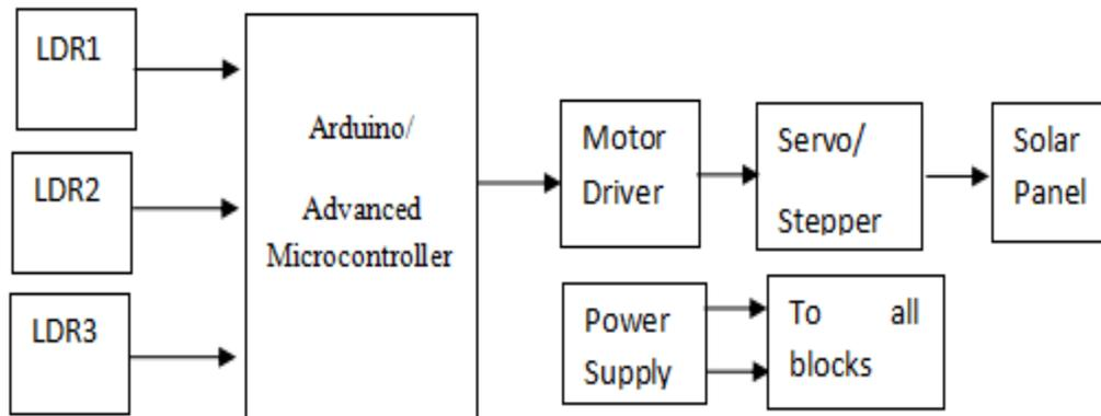
Figure 4: Block diagram of solar tracking system
