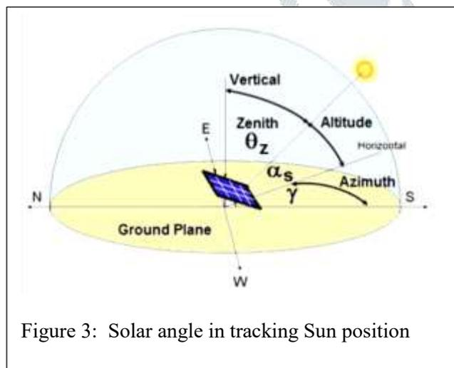
Figure 3: Solar angle in tracking Sun position
