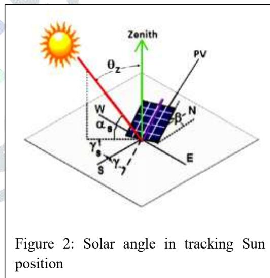
Figure 2: Solar angle in tracking Sun position
