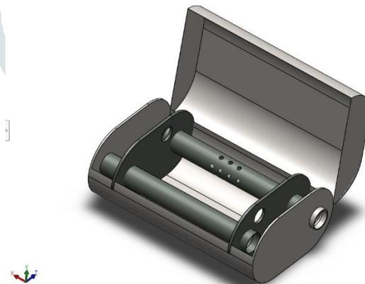
It is a CAD model which is done using the design software Solidworks 2018 version. We have used the assembly command to club various sections of this system. We have selected material for the model according to the real material specifications. For example - We have used Cast Iron material for pipes and partition and we have used Steel for shell, shell cover.
