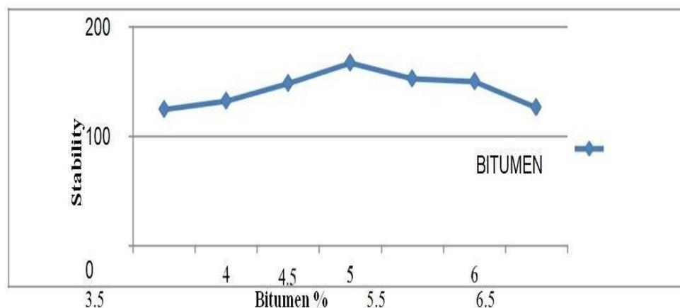
Fig. . Graphical representation of Marshall Stability value of bitumen without PET mix in it:
