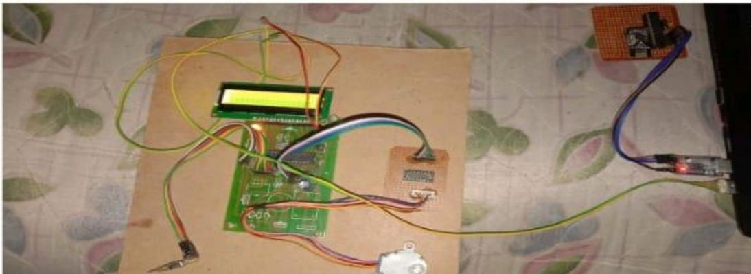
The stepper motor working principle is Electro-Magnetism. It includes a rotor which is made with a permanent magnet whereas a stator is with electromagnets. Once the supply is provided to the winding of the stator then the magnetic field will be developed within the stator. Now rotor in the motor will start to move with the rotating magnetic field of the stator. So this is the fundamental working principle of this motor.
