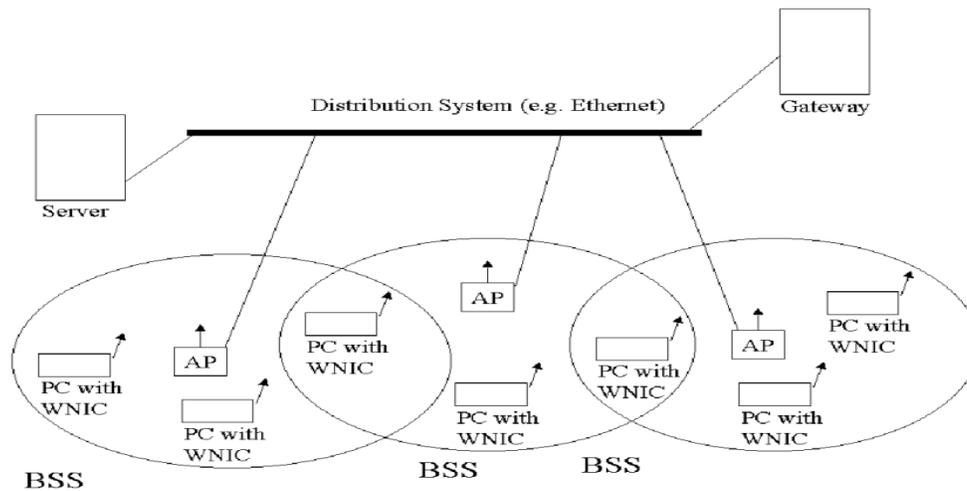
**Figure 4: Extended Service Set - ESS**
