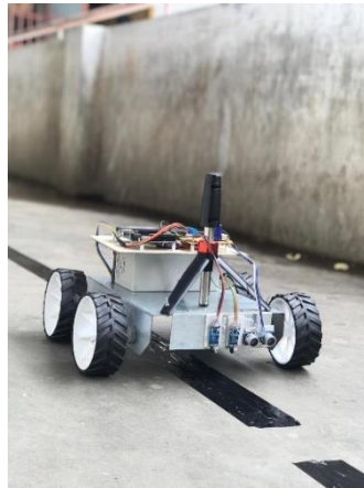
Fig 3 Robot tracking black line like AGV
