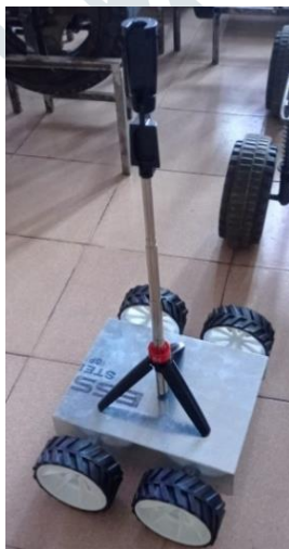
Fig 2 Tripod attached with chassis
