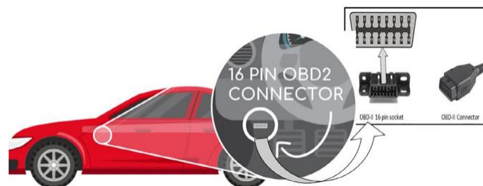
Figure: - OBD-II port in car (near driver wheel under dash board)
