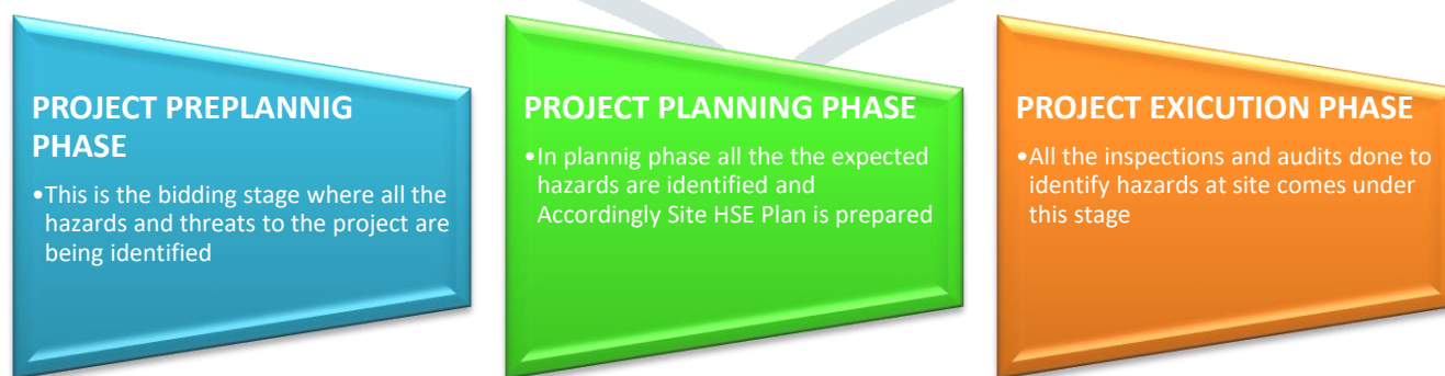
Figure 9- Stages of Hazard Identification at Construction Project
