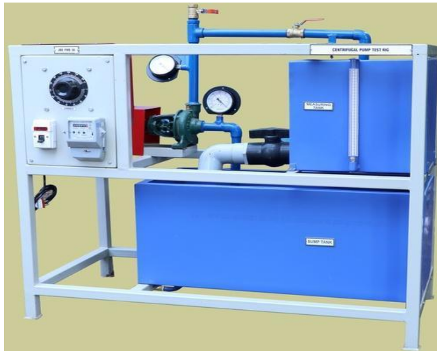
Figure : Set up of Centrifugal Pump Test Rig
