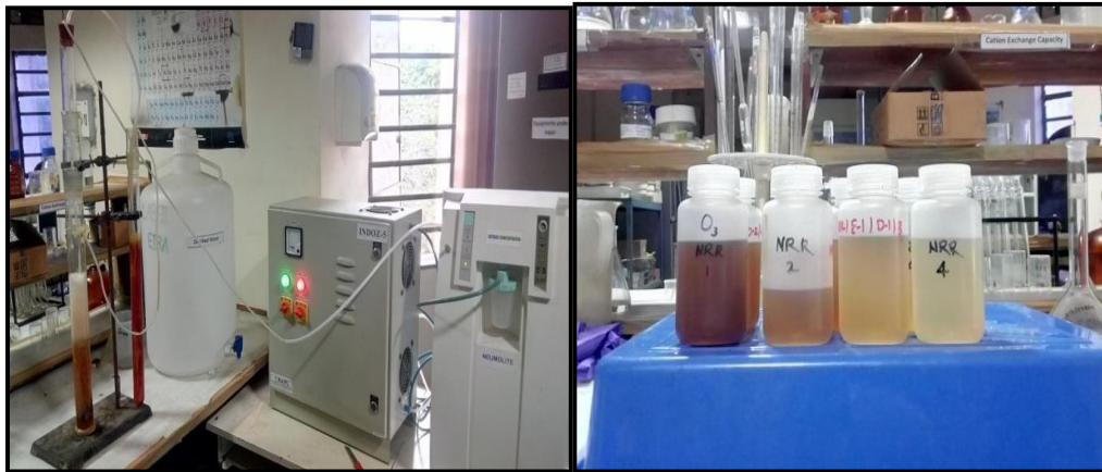
Figure 18: Ozonation studies at lab scale
