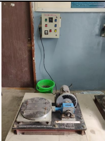
(Fig.2.1) Horizontal Shaking Machine
