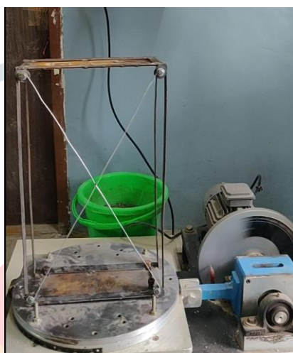
(Fig.2.4) Frame with x-wire bracing-Stable Condition
