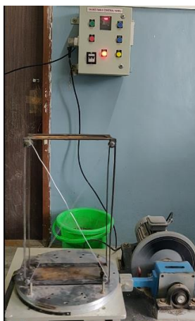
(Fig.2.5) Frame with x-wire bracing- Unstable Condition
