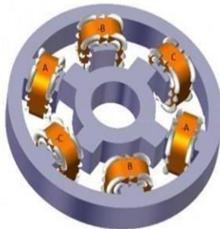
Fig 2: Inside Stepper motor coils
