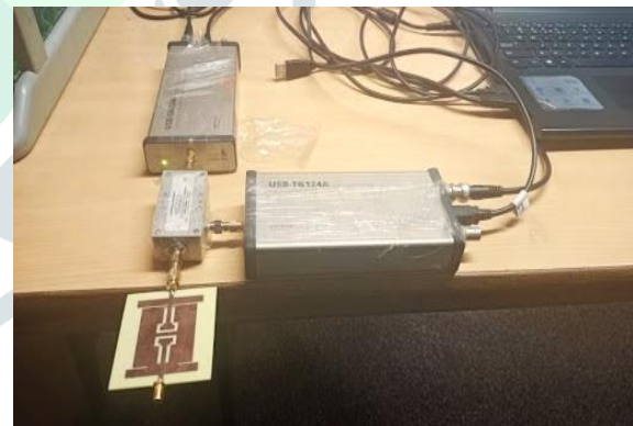
Fig 2.3: Testing of Fabricated Antenna
