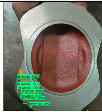
Figure 7. Defect detected image
