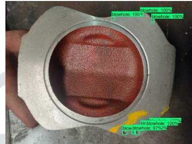
Figure 9. Defect detected image
