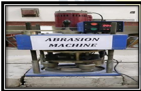
Fig. 2.8 Abrasion resistance test on concrete in slab
