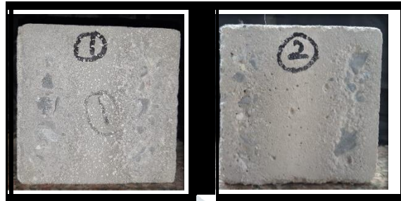
Fig. 2.12 Sample after Sand Blasting
