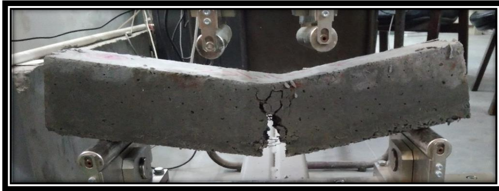
Fig. 2.6 Flexural strength test in progress
