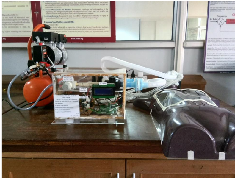
Figure. 10. Working Ventilator of Low-Cost Ventilator with Human lung model
