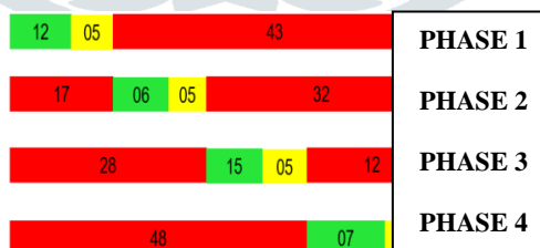
Figure No. 2.5 Final signal timing diagram
