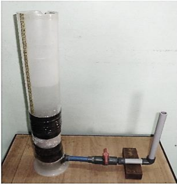
Figure 2. Experiment setup of permeability testing.
