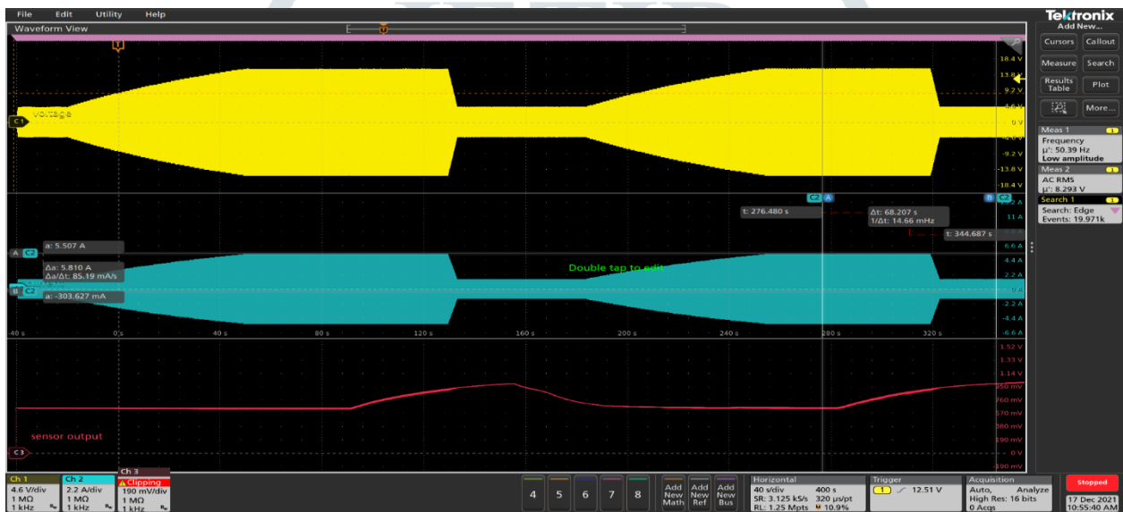
Fig-6 : Output voltage : Yellow, output current : Blue and Temperature sensor : Red at 28VDC for 3-ohm resistive load condition
