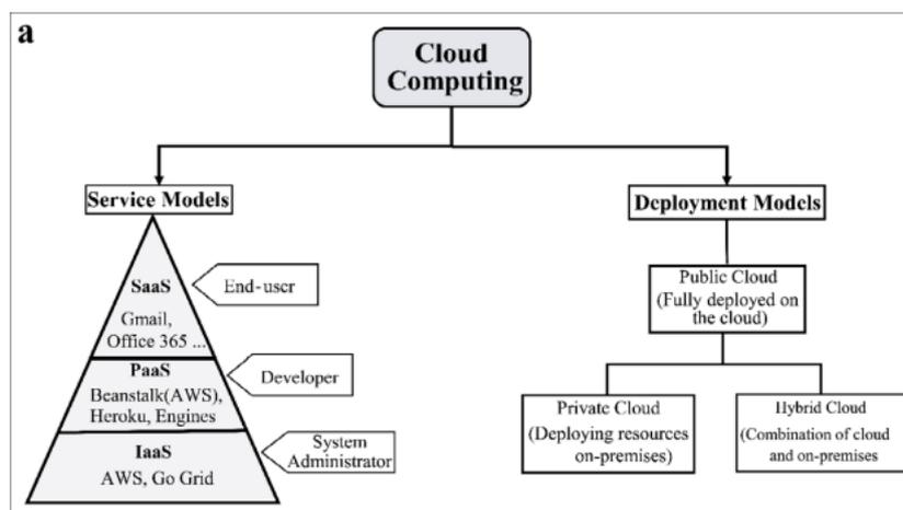
Figure 2 Cloud computing architecture
